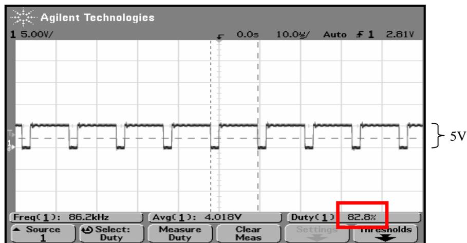
**Figure 11** Controller PWM signal
