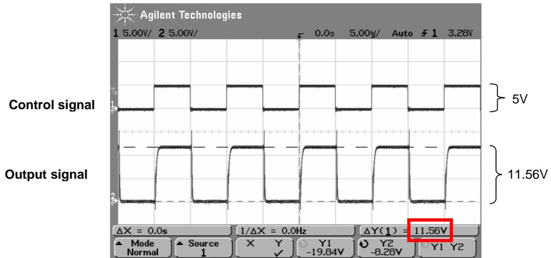
Figure 13 Control signal & IR2117 output ( $V_s$  ground)
