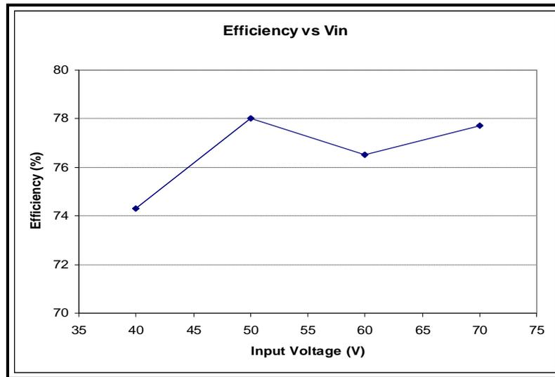
**Figure 16** Overall efficiency over input range
