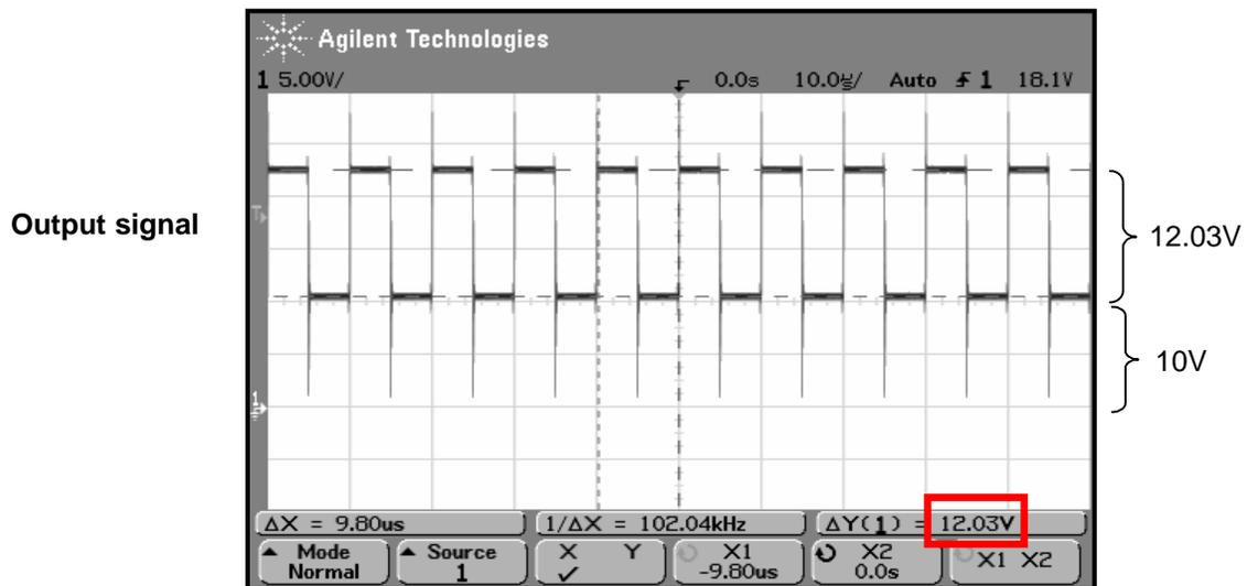
Figure 14 Control signal & IR2117 output ( $V_s = 5V$ )
