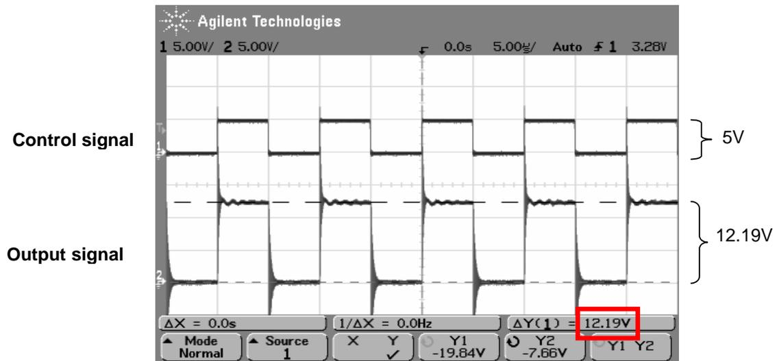
Figure 12 Input control signal & MIC4420 output
