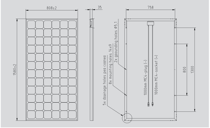
Dimensioned drawing STP180S-24/Ad, STP185S-24/Ad
