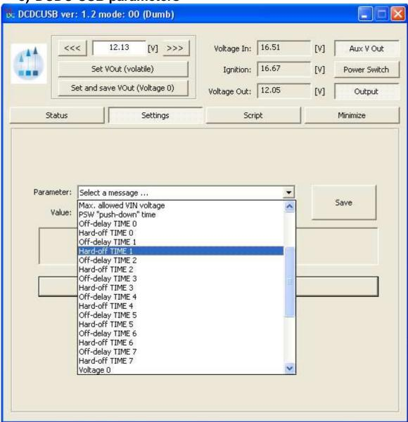
In this page you can see how several parameters can be configured by selecting it from the combo-box. After changing the value press the "Send" button to send it to the device. The parameter changed will have effect on the next power cycle.
