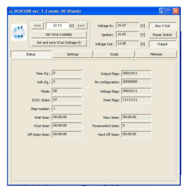
In this page you will find detailed description of several internal states and timers used in different modes: DUMB, AUTOMOTIVE, SCRIPT. Ex: this is useful when using the SCRIPT mode and testing the script programmed.
