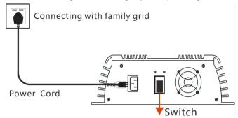
5. Switch on power grid after check for input and output connections are correct and then switch on the Smart Microinverter. The Red/green LED lights up at the same time and then red LED lights off follow on and green LED flash fast, it is means that Smart Microinverter is run for MPPT operation. When green LED long light and it is means that maximum power point lock-in, Smart Micro inverter proper functioning and output steady.
